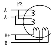
Figure 9: 8-lead motor parallel connections
