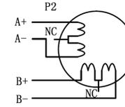
Figure 7: 6-lead motor full coil (higher torque) connections
