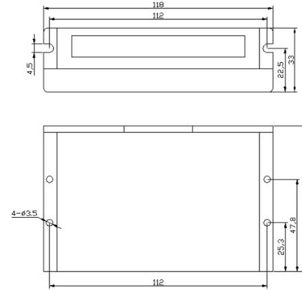
Figure 1: Mechanical specifications
