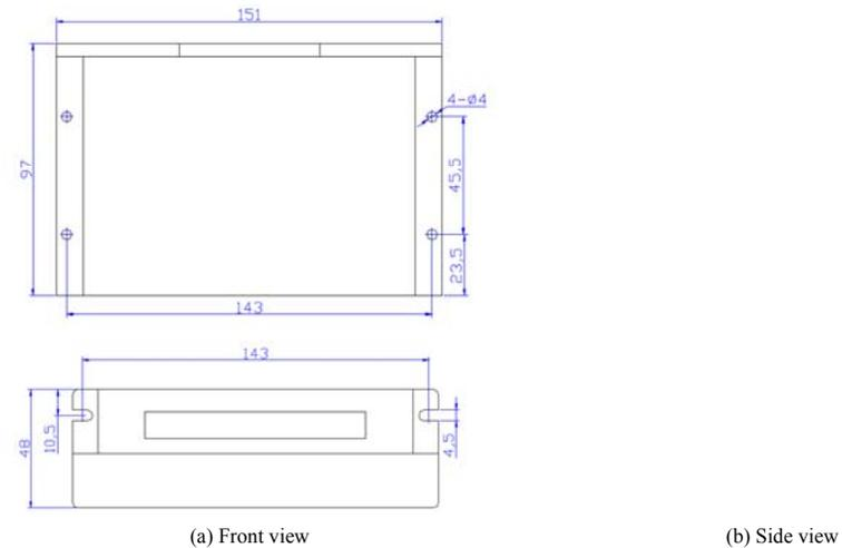
Figure 1: Mechanical specifications
