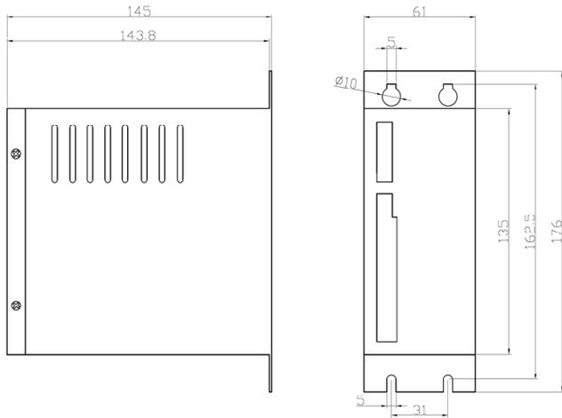
Figure 1: Mechanical specifications
